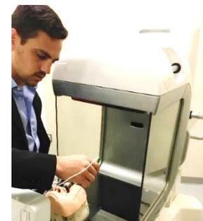
Figure 1: Experimental set-up showing the Xoran xCAT™ intraoperative CT scanner (right), Fiagon navigation system field generator (left), automatic registration device, located on phantom forehead.
